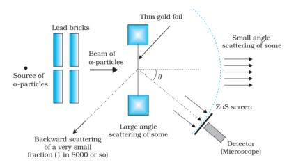
Schematic arrangement of the Geiger-Marsden experiment.co relates the two figures. A typical graph of the total number of  $\alpha$ -particles scattered at different angles, in a given interval of time, is shown in Figure
