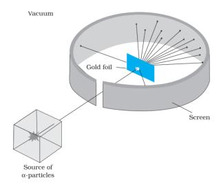
Geiger-Marsden scattering experiment. The entire apparatus is placed in a vacuum chamber (not shown in this figure)
